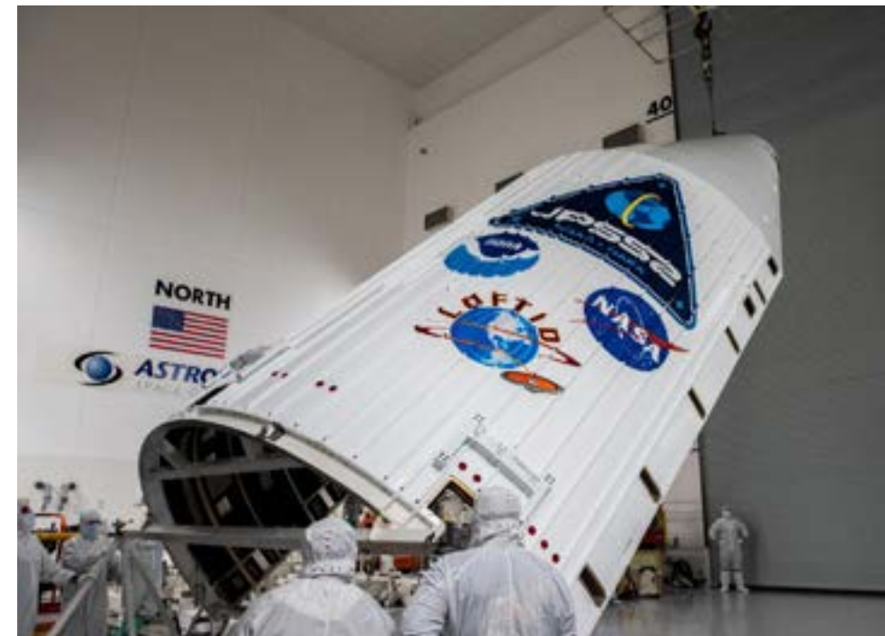
On August 11, 2022, teams at the VSBF Astrotech facility in California used a crane to raise to vertical one of the ULA Atlas V payload fairing halves for the JPSS-2 satellite mission. The payload fairing protects the spacecraft during launch and flight through the atmosphere. CREDIT: USSF 30TH SPACE WING/JULIO PAZ
