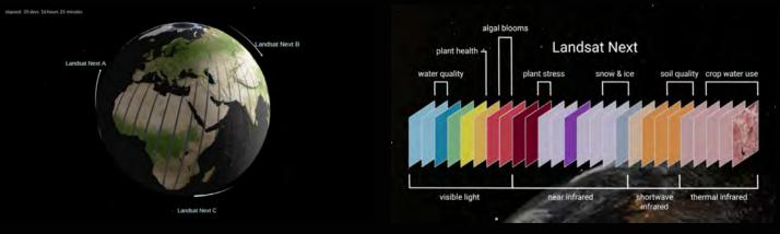
Landsat Next will be a trio of smaller satellites that can each detect 26 wavelengths of light and thermal energy. (top) Landsat Next will be "super-spectral" adding 15 new bands to support emerging user applications—for a total of 26 spectral bands. (bottom) CREDIT: NASA
