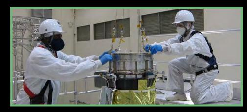
Lift and integration of the Resolve X-ray Mirror Assembly onto the top of the XRISM spacecraft at the Tsukuba Space Center in October 2022. From left: Marcellus Ajiboye and Steven Kenyon. CREDIT: NASA/JAXA
