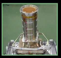
Xtend, an X-ray CCD camera that captures images over a wide wavelength range. CREDIT: JAXA
